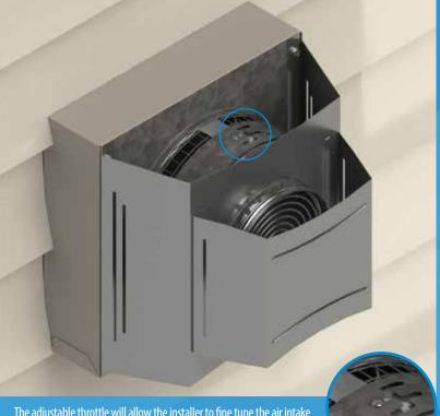
The adjustable throttle will allow the installer to fine tune the air intake to the appliance for the best looking flame possible. It can be adjusted to handle the dominate outside wind conditions.
